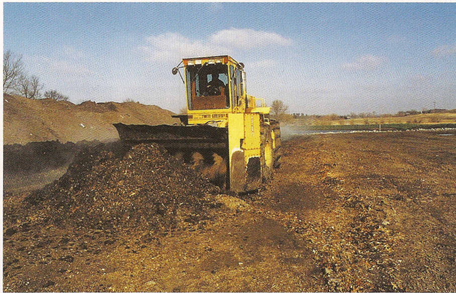
The Brown Bear's paddle style rotor mixes, aerates and turns the windrows.
