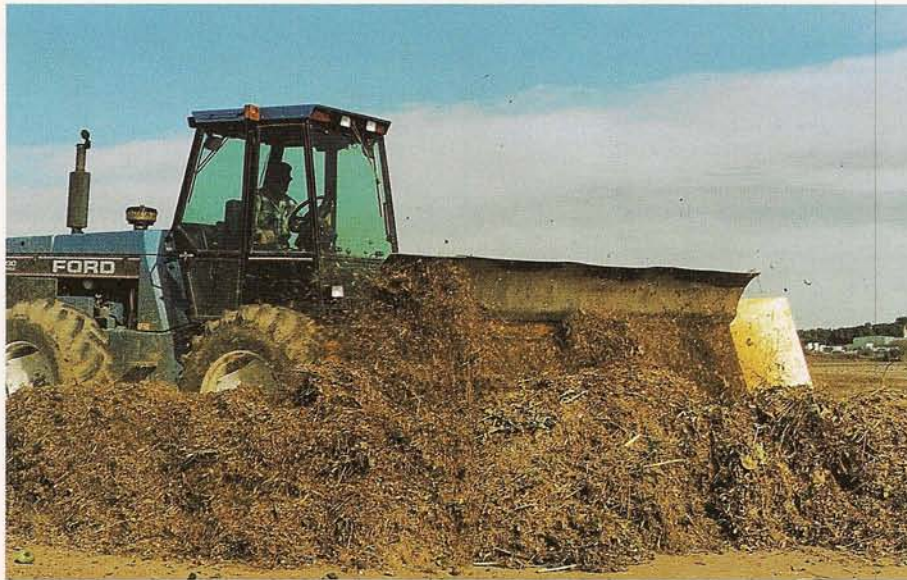
Paddle reduces particle size.
