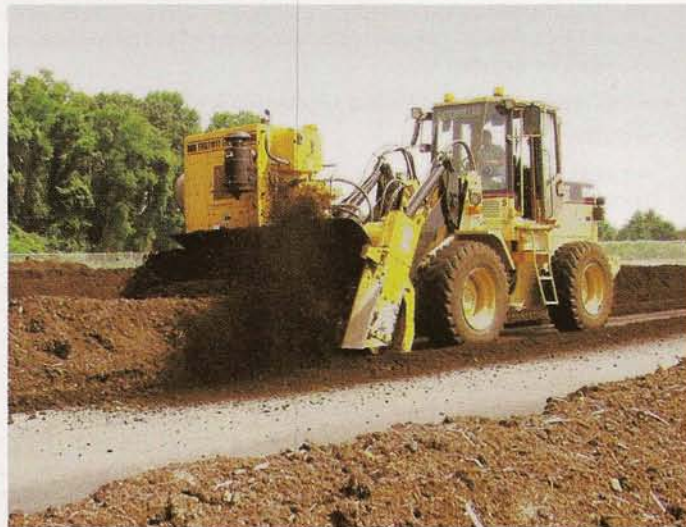
At the Pennsylvania site, the Township purchased a truck chassis with a hook-lift design for interchanging the leaf vacuum with the dump box (far left, left). Windrow turner (below) can place piles edge to edge after each pass.
