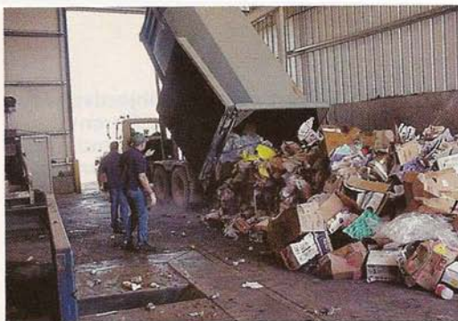
The composting plant in Nevada processes 10 tpd, with steps that include an MSW tipping floor (top), loading end for mixing vessels (center), and the final finishing building (bottom).
