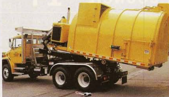
At the Pennsylvania site, the Township purchased a truck chassis with a hook-lift design for interchanging the leaf vacuum with the dump box (far left, left). Windrow turner (below) can place piles edge to edge after each pass.
