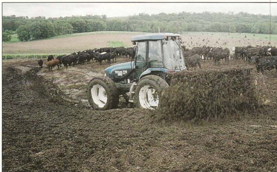
Summer and winter, Cold Springs Farm's unique tractor-mounted aerator compostor strips manure from its feeder pens without disturbing the clay base below.
