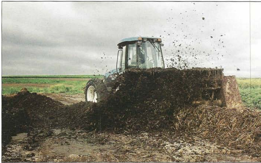
The versatile unit works within a composting area to mix the manure with hay, creating a seed-free pathogen-free, high-nutritive soil additive.
