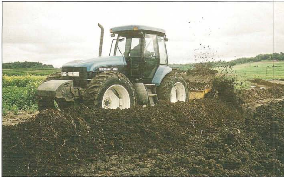
Windrows in the separate compost site are laid adjacent to one another to reduce the space requirement.
